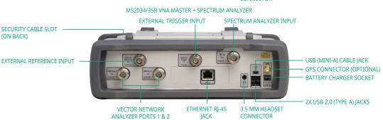
ALL CONNECTORS ARE CONVENIENTLY LOCATED ON THE TOP PANEL, LEAVING THE SIDES CLEAR FOR HANDHELD USE
